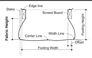
Using the edge line determined in step 2, staple corner edges to top of screed boards at 12" on center, using a hammer tacker with 3/8" staples.
