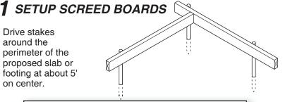
SOLIDLY ATTACH SCREED BOARDS Concrete produces downward tension in fabric. Use 3 nails or 2 screws (2-1/4") per stake.
