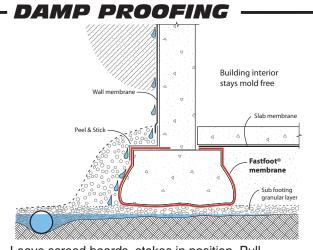
Leave screed boards, stakes in position. Pull Fastfoot® off screeds and tape two edges together on top of footing with 2" sheathing tape. Form and pour wall. After stripping (if required) run 12" width of peel & stick membrane along top of footing (covering staple holes in Fastfoot®) and up side of wall. Lap bottom edge of wall membrane over vertical peel & stick. On the inside, tape underslab membrane to interior Fastfoot®.
