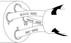
4. Tighten all the terminal screws to 25 in-lbs torque.
