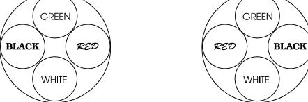
2. Insert the black and green wires into the "Y" and "G" terminals, and tighten the two terminal screws. **Note:** The drawing shows the plug. The "Y" terminal is on the other side on the connector.
