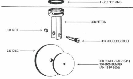
\*\*\*For Model AH-15-GL the four parts shown below line are replaced with the 300-01 Aluminum Piston and the 5/16-18 x 1-1/2" Screw
